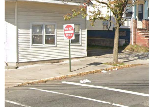
An extended tree pit, which is partially in the roadway and partially in the sidewalk, can be installed north of the intersection to capture, treat, and infiltrate the stormwater runoff from the roadway. A preliminary soil assessment suggests that more soil testing would be required before determining the soil's suitability for green infrastructure.
