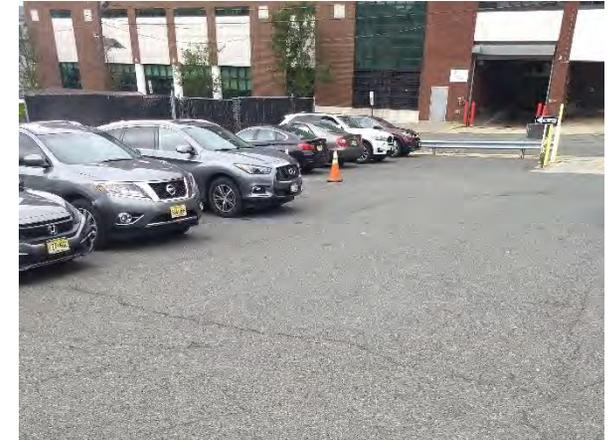
Parking spaces in the parking lots west and north of the building can be converted to porous pavement to capture and infiltrate stormwater runoff from the parking lots. Two rain gardens can be installed on either side of the front entrance to the administrative building located along the parking lot to the north of the medical center. A preliminary soil assessment suggests that more soil testing would be required before determining the soil's suitability for green infrastructure.
