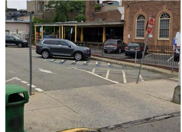
Western parking spaces in the parking lot can be converted to porous pavement to capture and infiltrate stormwater runoff from the parking lot. A preliminary soil assessment suggests that more soil testing would be required before determining the soil's suitability for green infrastructure.
