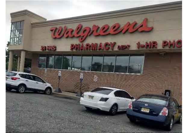
Parking lot spaces to the east and west of the building can be converted to pervious pavement to capture and infiltrate the stormwater runoff from the parking lot. A preliminary soil assessment suggests that more soil testing would be required before determining the soil's suitability for green infrastructure.
